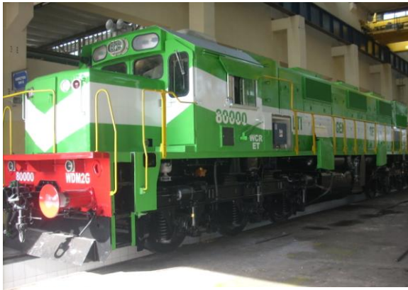
Manufacture of 1st Multi Gen Set Loco
