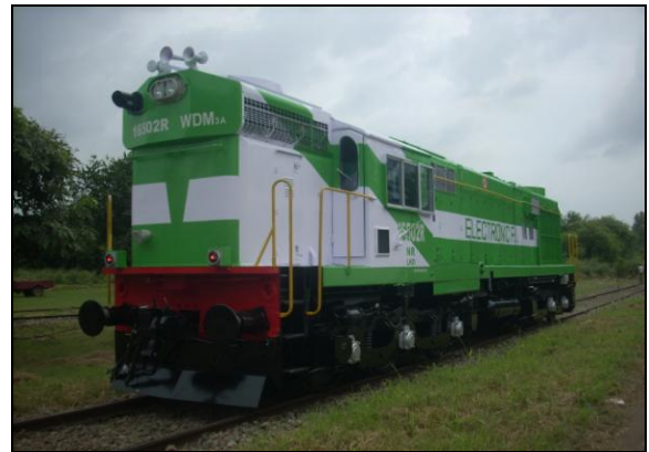
EFI fitted Locomotive
