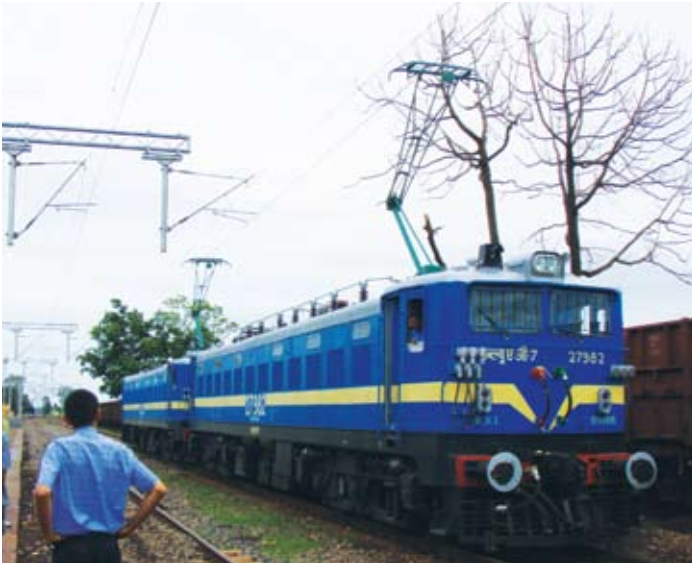
Two WAG-7 locomotives were fitted with high-reach pantographs for the trials.
